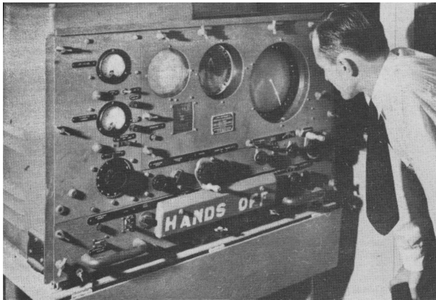
The radar console of Isbrandtsen Lines' S.S. Flying Clipper . Many freighters are already equipped with this great aid to navigation that can "see" through fog.
